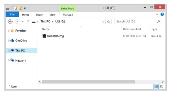
1. Place the updated software file in the empty USB drive, which is to avoid the conflict between the updated software file and other files in the USB drive. The updated software file is the only file that should be on the USB drive.
