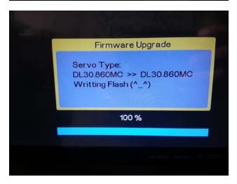
4. After MCU update, the unit will turn off, at this point press the reset button for 10 seconds then restart the unit.(Reset button is the small pin hole on the front face of the unit)
