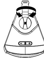
The silicon carry-strap is removable by untwisting the thumb screw.
