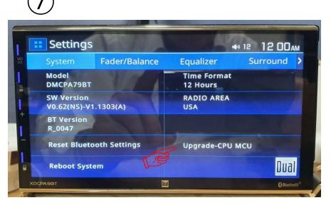
Move to Setting Mode Screen and press Upgrade-CPU MCU Text for over 3 seconds.
