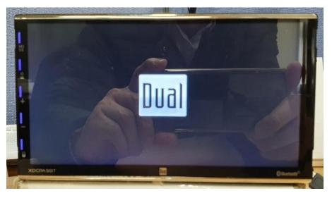
Power off / on automatically when MCU and CPU firmware is completed.
