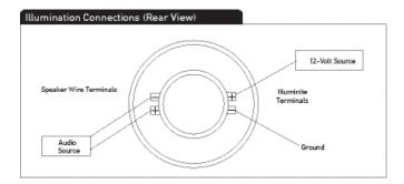
**Note:** The Illuminite series LED illumination elements are not removable. There are no serviceable parts inside or attached to the speaker assembly. The Illuminite series products are sensitive electronic devices. Removal or tampering with any part or portion of the speaker and/or its assemblies will damage the product and void the limited warranty.
