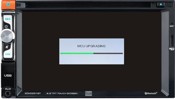
7. Once the update is complete you will see the below screen. Remove the USB thumb drive and turn your vehicle off and then back on. This will complete the MCU update.
