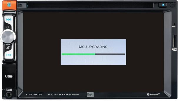
7. Once the update is complete you will see the below screen. Remove the USB thumb drive and turn your vehicle off and then back on. This will complete the CPU update.
