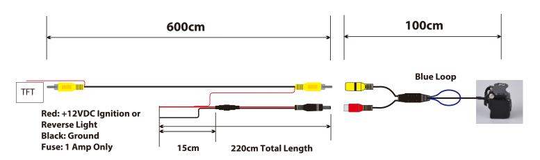
Note: Video cable has a built-in power wire (2 red wires on either end) for ease of installation. Only 1 cable has to be routed during installation.
