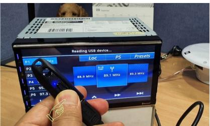
Insert USB Thumb Drive with Update Firmware into DMCPA9BT's USB Port.
