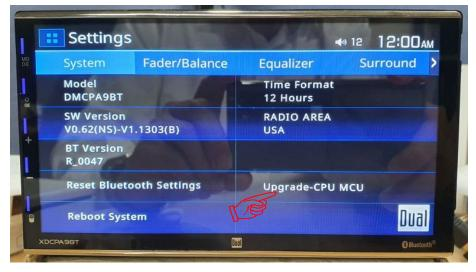
Move to Setting Mode Screen and press Upgrade-CPU MCU for 3 seconds.
