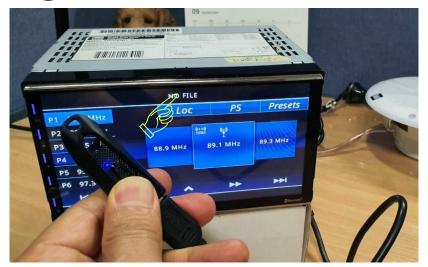
NO FILE Text is displayed while checking the Update Firmware on the USB.
