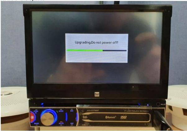
7. 7. When the update is completed, the TFT LCD Panel is closed as shown below. Remove the USB thumb drive and turn the vehicle off and on again. This completes the CPU update.
