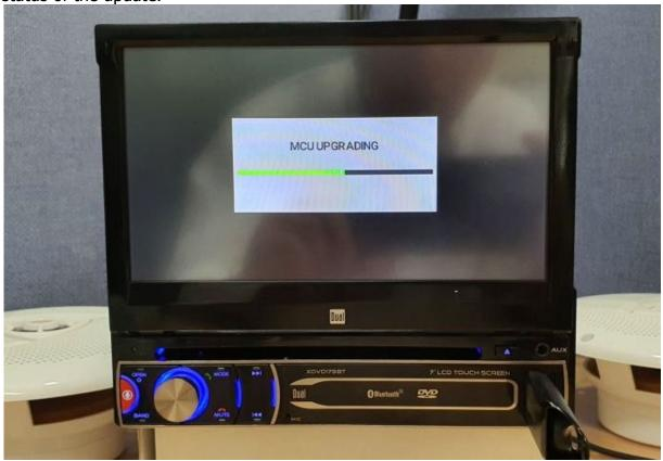
7. Once the update is complete you will see the below screen. Remove the USB thumb drive and turn your vehicle off and then back on. This will complete the MCU update.
