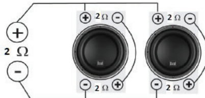
(2) 2ohm DVC Speaker = 2 ohm Load
