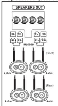
Typical Stereo Wiring
