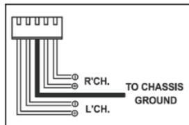
**Note:** Do not use both low and high level inputs at the same time - connect only one or the other.
