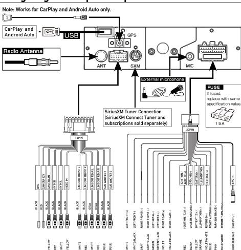
When replacing a fuse, make sure to use the correct type and amperage. Using an incorrect fuse could cause damage. The unit uses (1) 15 amp ATC mini style fuse located on the power connector.
