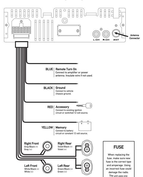
10 amp ATC fuse located beside the wiring connector.
