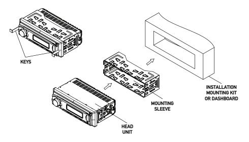
TYPICAL FRONT-LOAD DIN MOUNTING METHOD
