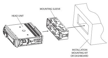
TYPICAL FRONT-LOAD DIN MOUNTING METHOD
