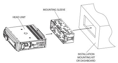
TYPICAL FRONT-LOAD DIN MOUNTING METHOD
