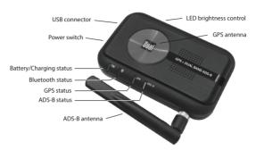
Please refer to the diagram above to locate the controls and indicators on the XGPS170D.
