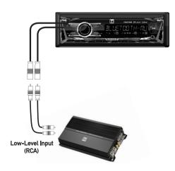
**Note:** Do not use both low and high level inputs at the same time - connect only one or the other.
