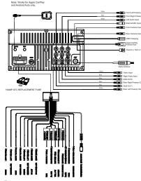
Note: When replacing a fuse, make sure to use the correct type and amperage. Using an incorrect fuse could cause damage. The unit uses (1) 15 amp ATC mini style fuse located on the power connector.
