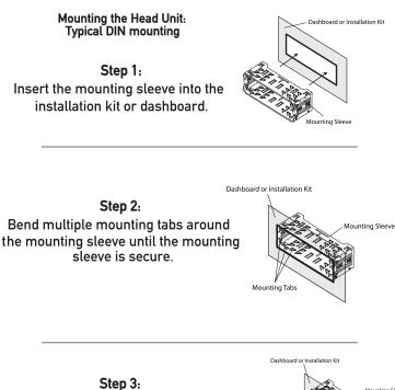
Connect all wiring harnesses and slide the head unit into the mounting sleeve until it clicks into place.
